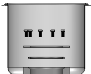
Stainless Steel Containment Vessel Stainless Steel Bolts Flange O-ring Seal
