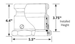
The Emco Wheaton A0030-124S Swivel Fill Adapter typically installs on the tank fill riser. The top of the adapter rotates 360 degrees while the base is stationary, preventing accidental loosening from the riser during fuel deliveries. The A0030-124S is *field serviceable* using the kits below. Use with the A0097 Fill Cap. Use the Emco Wheaton A0081-001 Adapter Wrench for installation and removal.
