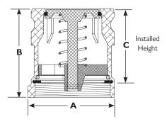
The Emco Wheaton A0076 Vapor Adapter is used in dual point fill systems on the vapor return line. It features a poppet design which seals off the vapor path and external lugs on the adapter body for easy installation. Use with the A0099-002 Vapor Cap.
