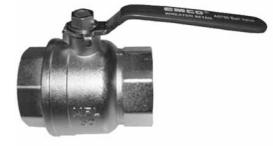
The Emco Wheaton A0750 Ball Valve is a full port 2" valve. Thread depth is .865"; inside diameter is 2". 150 psi working pressure.
