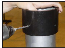
566675, 572719 Drill Fixture Aligns holes for attaching support collar
