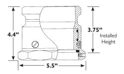
The Emco Wheaton A0030-124S Swivel Fill Adapter typically installs on the tank fill riser. The top of the adapter rotates 360 degrees while the base is stationary, preventing accidental loosening from the riser during fuel deliveries. The A0030-124S is *field serviceable* using the kits below. Use with the A0097 Fill Cap. Use the Emco Wheaton A0081-001 Adapter Wrench for installation and removal.
