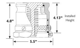
The Emco Wheaton A0076-124S Vapor Swivel Adapter typically installs on the tank vapor riser. The top of the adapter rotates 360 degrees while the base is stationary, preventing accidental loosening from the riser during fuel deliveries. A normally closed poppet valve opens to recover the vapor. The A0076-124S is *field serviceable* using the kits below. Use with the A0099-002 Vapor Cap. Use the Emco Wheaton A0081-001 Adapter Wrench for installation and removal.
