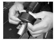
6. Install the new boot face into the boot connector by pressing evenly. Align the four mounting holes of the boot face with those of the boot connector.
