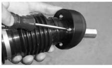
4. Use the philips screw driver to remove the four mounting screws located on the back of the boot connector.
