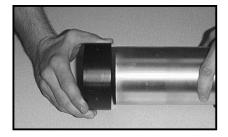
5. Slide the EMCO Drill Fixture p/n 566675 onto the end of the top drop tube until the edge bottoms out against the inside ridge.
