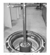
Step 4: Use the EMCO Adapter Wrench p/n A0081-001C to loosen and remove the A0076-124S swivel vapor adapter.
