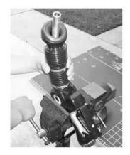
It is unnecessary to remove the A4005EVR nozzle from the fueling point during the removal and installation of the bellows and boot face. Use the bench vise to properly secure the A4005EVR nozzle during service.
