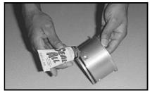
10. Apply a 1/2 inch bead of Seals-All sealant around the o-ring and outside area of the A1100EVR collar. Verify the o-ring is properly secured inside the machined groove.
