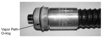
Before attempting to install the A4005EVR nozzle onto the curb hose, verify the vapor path o-ring is properly secured onto the connector, and in good working condition. Lightly lubricate the o-ring using petroleum jelly or other suitable lubricant.
