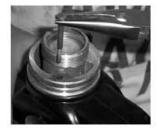
13. Use the needle nose pliers to install the new interlock push rod.
