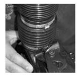
11. Use the bellows band clamp crimp tool p/n 494652EVR to crimp and secure into place.
