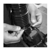
5. Locate the bottom bellows band clamp. Use the flat head screw driver to dislodge the locking mechanism and remove the band clamp from the bellows.
