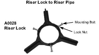
IMPORTANT: All <u>single wall configurations</u> come standard from the factory with one A0028 riser lock. The purpose of the A0028 riser lock is to prevent the riser pipe from turning during removal and installation of the primary liner.
