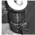
24. Use the bellows band clamp crimp tool p/n 494652EVR to crimp 7 and secure into place.
