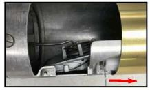
**Step 6:** Using a scribe move the primary float upward to unlatch the flapper valve, and with the hook end secured, gently tug on the test tool, the flapper valve must close, the test tool will move about 3" downward. *Refer to Figures 5, 6, 7 and 8 for details.*
