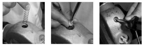
11. Remove the A4005EVR nozzle from the bench vise and turn top side up. Install the existing spring around the square stem. Fasten the existing brass screw by hand onto the top of the square stem to avoid cross threading. Use the flat head screw driver to tighten.
