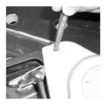
Remove the A4005EVR nozzle from the bench vise and place on a flat surface. Use the 1/8" diameter punch and hammer to lightly tap and remove both mounting rivets located on the lever guard.
