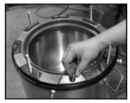
**Step 8:** Loosely install four of the eight 3/8" bolts into the open holes on the spill containment plow ring.
