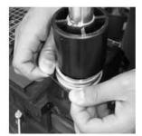
19. Install the new bellows o-ring. Verify that the o-ring seats properly into the machined groove.
