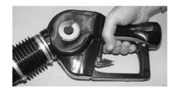
19. Functional test the insertion interlock of the A4005EVR nozzle by compressing the bellows and then squeezing the lever. The A4005EVR nozzle will not function unless the insertion interlock is properly engaged.
