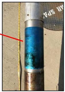
**Figure 1:** Correct position, primary float facing downward.
