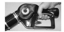
14. Functional test the insertion interlock of the A4005EVR nozzle by compressing the bellows and then squeezing the lever. The A4005EVR nozzle will not function unless the insertion interlock is properly engaged.
