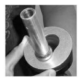
21. Use the bellows retainer plate tool p/n 494712EVR to secure and lock the bellows and boot face in place.
