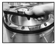
**Step 10:** Remove the four studs and discard. Install the four remaining 3/8" bolts. In a star pattern tighten and torque all eight 3/8" bolts to 20 ft-lbs.
