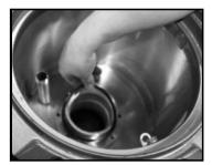
Step 10: Install the new o-ring over the female coupling. Push downward until the o-ring is properly seated in the o-ring groove of the flange assembly.
