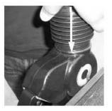
10. Slide the new bellows over the spout until the end reaches the nozzle body. Push down over the bellows o-ring until properly seated.
