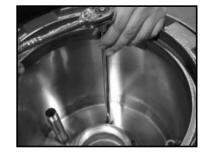
**Step 14:** In a star pattern tighten and torque all eight 9/16" flange bolts to 15 ft-lbs., and re-install EZ-Gage.
