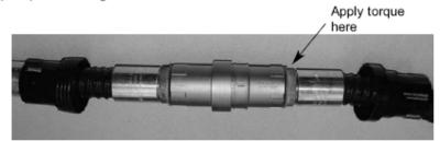
9. Using a 1 7/8" crows foot and torque wrench, tighten the curb hose connector to 50 ft-lbs of torque.
