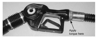
Using a 1 7/8" crows foot and torque wrench tighten the curb hose connector to 50 ft-lbs of torque.
