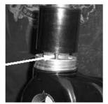
8. Before attempting to install the new bellows and boot face verify that the top of the interlock push rod is properly aligned with the bottom edge of the interlock guide.
