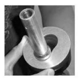
11. Use the bellows retainer plate tool p/n 494712EVR to secure and lock the bellows and boot face in place.
