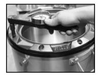
**Step 9:** Remove the four studs and discard. Install the four remaining 3/8" bolts. In a star pattern tighten and torque all eight 3/8" bolts to 20 ft-lbs.
