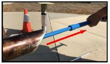
**Step 5:** With the flapper valve latched open, and the hook end secured, gently tug on the test tool, the flapper valve must remain open.
