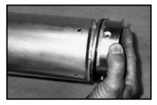
11. Slide the A1100EVR collar inside the top end of the drop tube and align the four holes.
