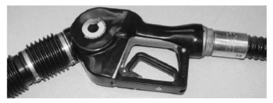
It is necessary to remove the A4005EVR nozzle from the curb hose during the removal and installation of the latch. Use the pipe wrench with flat jaws to loosen the curb hose connector. Unfasten the curb hose connector by hand from the A4005EVR nozzle to avoid cross threading.
