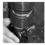
16. Use the bellows band clamp crimp tool p/n 494652EVR to crimp and secure into place.
