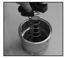
3. Remove the poppet guide and poppet spring from within the vapor top of the swivel adapter.
