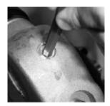
Install the new dust plug. Use the 5/8 punch and hammer to light tap into place.
