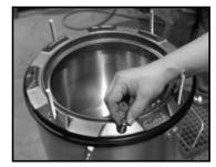
**Step 9:** Loosely install four of the eight 3/8" bolts into the open holes on the spill containment plow ring.
