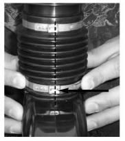
10. Install the new bottom bellows band clamp into the groove of the bellows. Lock and align the crimp portion with the parting line of the bellows.
