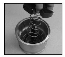
7. Re-install the poppet guide and poppet spring onto the stem of the vapor poppet which is located inside the vapor top of the swivel adapter.
