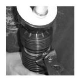
14. Use the bellows band clamp crimp tool p/n 494652EVR to crimp and secure into place.
