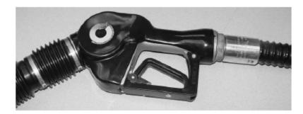
It is necessary to remove the A4005EVR nozzle from the curb hose during the removal and installation of the scuff guard. Use the pipe wrench with flat jaws to loosen the curb hose connector. Unfasten the curb hose connector by hand from the A4005EVR nozzle to avoid cross threading.
