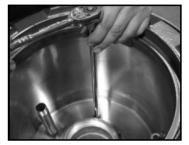
Step 13: In a star pattern tighten and torque all eight 9/16" flange bolts to 15 ft-lbs.
