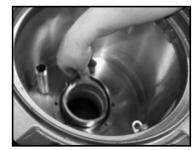
Step 11: Install the new o-ring over the female coupling. Push downward until the o-ring is properly seated in the o-ring groove of the flange assembly.
