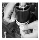
9. Install the new bellows o-ring. Verify that the o-ring seats properly into the machined groove.
