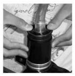
16. Install the new interlock guide by sliding the top and bottom pieces over the spout. Press the top piece into the bottom piece.
