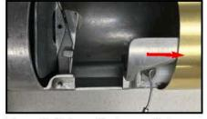
Figure 8: Primary float upward, flapper valve unlatched and closed.
