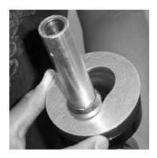
6. Use the bellows retainer plate tool p/n 494712EVR to secure and lock the bellows and boot face in place.
