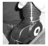
20. Slide the bellows over the spout until the end reaches the nozzle body. Push down over the bellows o-ring until properly seated.
