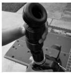
6. Remove the bellows and boot face from the A4005EVR nozzle. Grab the bellows and pull away from the nozzle body.
