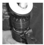
9. Use the bellows band clamp crimp tool p/n 494652EVR to crimp and secure into place.
