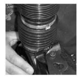
26. Use the bellows band clamp crimp tool p/n 494652EVR to crimp and secure into place.
