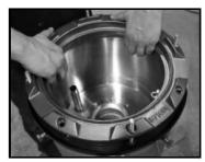
**Step 4:** Remove the spill containment plow ring and the primary insert by slowly pulling upward.
