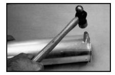
12. Using the indenter tool and a hammer, apply a sharp blow to counter sink each individual hole before attempting to install the mounting rivets.
