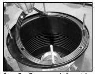
**Step 7:** Remove and discard the existing plow ring gasket. Install the new plow ring gasket, use the studs for alignment.
