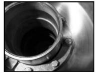
Step 13: Use the eighth 9/16" flange bolt and washer to install the new grounding clip. Be sure the grounding clip touches the female coupling.
