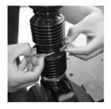
4. Locate the top bellows band clamp. Use the flat head screw driver to dislodge the locking mechanism and remove the band clamp from the bellows.
