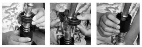
9. Disassemble the interlock guide. Remove the top piece by pulling upward and sliding over the spout. Remove the bottom piece by sliding over the spout.
