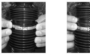
Install the new top bellows band clamp into the groove of the bellows. Lock and align the crimp portion with the parting line of the bellows.
