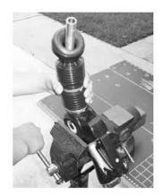
3. It is unnecessary to remove the A4005EVR nozzle from the fueling point during the removal and installation of the bellows band clamps. Use the bench vise to properly secure the A4005EVR nozzle during service.
