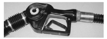
3. It is necessary to remove the A4005EVR nozzle and A4119EVR safe break valve from the curb hose during the removal and installation of the fuel path o-rings. Use the pipe wrench with flat jaws to loosen the curb hose connector. Unfasten the curb hose connector by hand from the A4005EVR nozzle to avoid cross threading.
