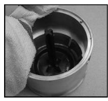
5. Clean and remove all existing grease, dirt, debris, etc. from the inside of the fill top and the outside of the base.
