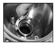
Step 11: Install the split flanges using seven of the eight 9/16" flange bolts.
