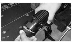
5. Remove the existing boot face by pulling out of the boot connector.
