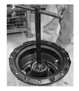
Step 5: Use the EMCO Adapter Wrench p/n A0081-001C to loosen and remove the A0030-124S swivel fill adapter.
