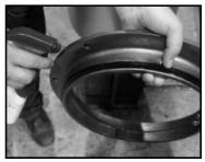
Step 6: Use a flat head screwdriver to remove the triple wiper seal from the bottom side of the spill containment plow ring. Install the new triple wiper seal and lubricate the outer wipers using heavy grease.
