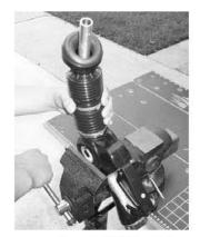
3. It is unnecessary to remove the A4005EVR nozzle from the fueling point during the removal and installation of the spout. Use the bench vise to properly secure the A4005EVR nozzle during service.
