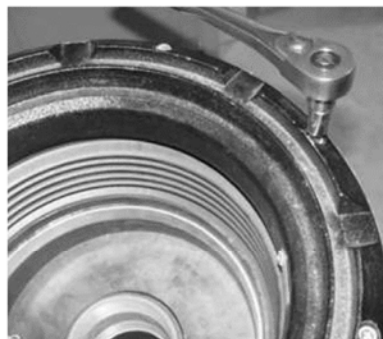
Step 6: Use a ratchet with a 3/8" socket or 1/4" allen wrench to remove and discard all eight 3/8" stainless steel bolts located along the top of the rim of the A1004EVR spill containment.
