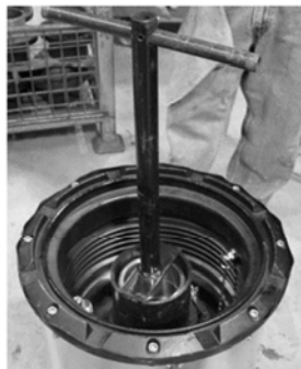
Step 5: Use the EMCO Adapter Wrench p/n A0081-001C to loosen and remove the A0030-124S swivel fill adapter.
