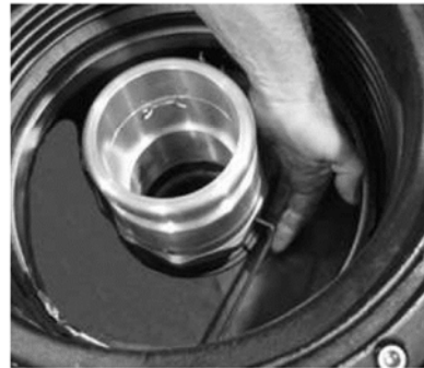
Step 4: Use a 5/32" allen wrench to loosen and remove both set screws from the base of the A0030-124S swivel fill adapter
