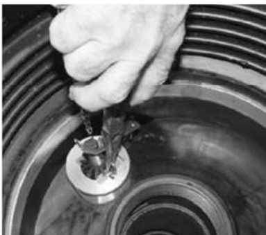
Step 3: Locate the 494118 drain valve. Begin by disassembling the pull chain and linkage. Use a pair of needle nose pliers to remove both cotter pins from the top, then lift and remove the filter.
