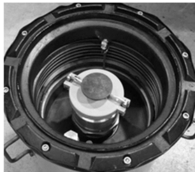
Step 2: Remove the A0097-005 fill adapter cap and dipstick.
