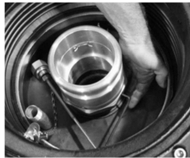
Step 4: Use a 5/32" allen wrench to loosen and remove both set screws from the base of the A0030-124S swivel fill adapter.
