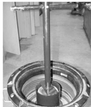
Step 4: Use the EMCO Adapter Wrench p/n A0081-001C to loosen and remove the A0076-124S swivel vapor adapter.
