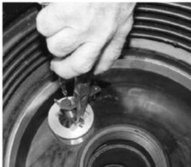
Step 3: Locate the 494118 drain valve. Begin by disassembling the pull chain and linkage. Use a pair of needle nose pliers to remove both cotter pins from the top, then lift and remove the filter.
