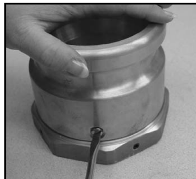
8. Re-install all three stainless steel screws to the base of the swivel adapter.
