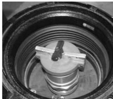
Step 2: Remove the A0099-002, -003 vapor adapter cap.
