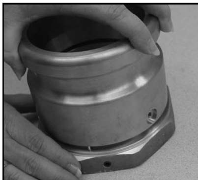
7. Reassemble the swivel adapter by placing the fill top over the base. Rotate and push downward slowly until both pieces bottom out.
