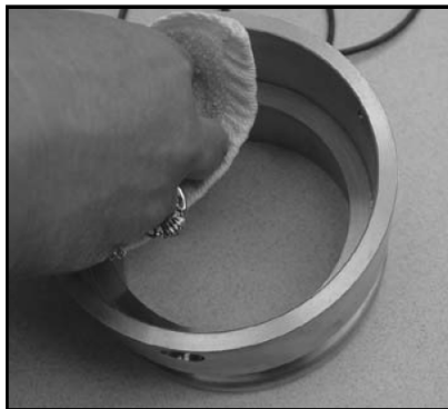
5. Clean and remove all existing grease, dirt, debris, etc. from the inside of the fill top.
