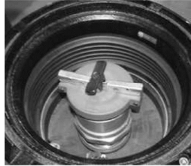
Step 2: Remove the A0099-002, -003 vapor adapter cap.
