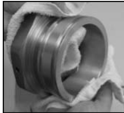
4. Clean and remove all existing grease, dirt, debris, etc. from the outside of the base.
