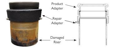
The Riser Repair Adapter installs on corroded/damaged 4" NPT threads to provide undamaged 4" NPSM threads for a product adapter. Three set screws hold the Repair Adapter onto the damaged pipe.
