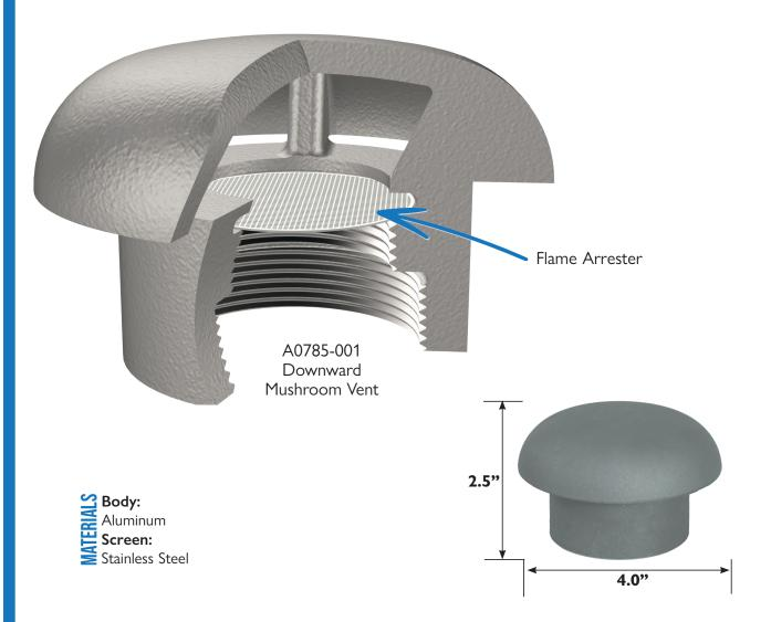
The Emco Wheaton A0785 Downward Mushroom Vent is designed for downward venting of storage tanks. The 30 mesh stainless steel screen can be easily removed for cleaning. A0785 threads onto either 1.5" or 2.0" vent lines. Clear coated aluminum for corrosion-free devices.
