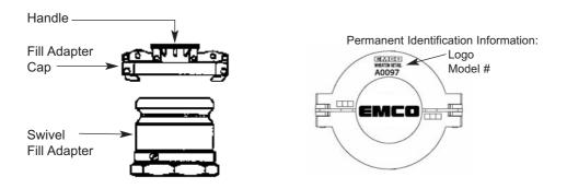
1. Locate the fill adapter cap over the swivel fill adapter and lock into place by pressing down on the handle.
