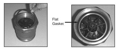
3. Remove the existing flat gasket and replace with new.
