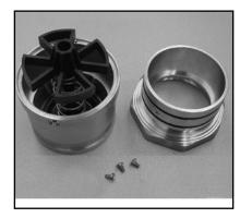
2. Separate the vapor top from the base of the swivel adapter by slowly rotating and pulling upward.
