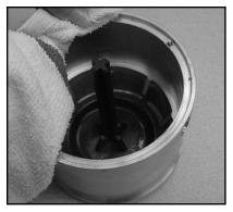
5. Clean and remove all existing grease, dirt, debris, etc. from the inside of the fill top and the outside of the base.
