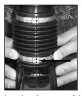
15. Install the new bottom bellows band clamp into the groove of the bellows. Lock and align the crimp portion with the parting line of the bellows.
