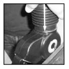
Slide the new bellows over the spout until the end reaches the nozzle body. Push down over the bellows o-ring until properly seated.
