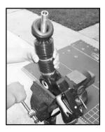
It is unnecessary to remove the A4005EVR nozzle from the fueling point during the removal and installation of the bellows and boot face. Use the bench vise to properly secure the A4005EVR nozzle during service.
