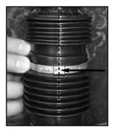
13. Install the new top bellows band clamp into the groove of the bellows. Lock and align the crimp portion with the parting line of the bellows.
