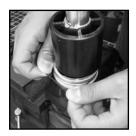
9. Install the new bellows o-ring. Verify that the o-ring seats properly into the machined groove.
