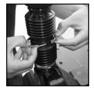
Locate the top bellows band clamp. Use the flat head screw driver to dislodge the locking mechanism and remove the band clamp from the bellows.
