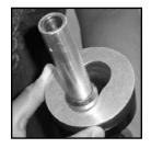
11. Use the bellows retainer plate tool p/n 494712EVR to secure and lock the bellows and boot face in place.
