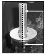
12. Slowly rotate the bellows until the parting line of the boot connector is aligned with the spout and automatic shut-off.
