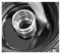
Step 4: Use a 5/32" allen wrench to loosen and remove both set screws from the base of the A0030-124S swivel fill adapter
