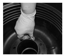
Step 4: Install the new bolts and washers to the bottom of the new secondary unit. Use a ratchet with a 5/16" allen wrench socket to tighten and torque to 40 ft-lbs.
