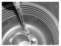
Step 1: Use a ratchet with a 5/16" allen wrench socket to remove the bolts and washers from the bottom of the secondary unit. Use a flathead screwdriver to pry the flange away. Set the flange aside and discard the bolts and washers. Remove secondary unit from the inside of the A1004EVR spill containment and discard.
