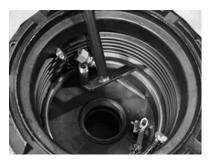
Step 10: Use the EMCO Spill Containment Wrench p/n A0081-001H to loosen and remove the primary unit from the secondary.
