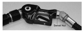
3. It is necessary to remove the A4005EVR nozzle from the A4110EVR hose swivel during the removal and installation of the vapor path o-ring. Use the pipe wrench with flat jaws to loosen the swivel nut. Unfasten the swivel nut by hand from the A4005EVR nozzle to avoid cross threading.
