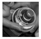
8. Lightly lubricate the vapor path o-ring using petroleum jelly or other suitable lubricant.
