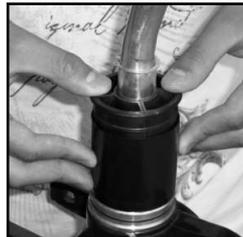
16. Install the new interlock guide by sliding the top and bottom pieces over the spout. Press the top piece into the bottom piece.
