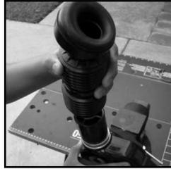
6. Remove the bellows and boot face from the A4005EVR nozzle. Grab the bellows and pull away from the nozzle body.
