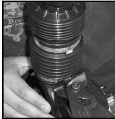
26. Use the bellows band clamp crimp tool p/n 494652EVR to crimp and secure into place.
