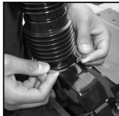
5. Locate the bottom bellows band clamp. Use the flat head screw driver to dislodge the locking mechanism and remove the band clamp from the bellows.
