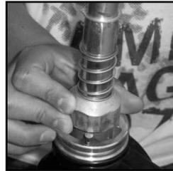
10. Use the 15" crescent wrench to loosen the spout nut. Unfasten the spout nut by hand to avoid cross threading.
