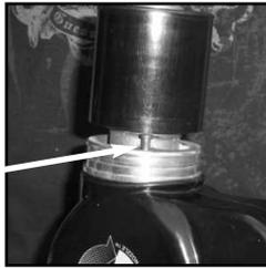
18. Before attempting to install the existing bellows & boot face verify that the top of the interlock push rod is properly aligned with the bottom edge of the interlock guide.
