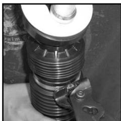
24. Use the bellows band clamp crimp tool p/n 494652EVR to crimp and secure into place.
