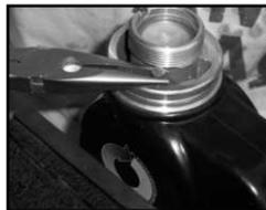
12. Use the needle nose pliers to remove the interlock push rod.
