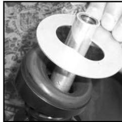
27. Remove the bellows retainer plate tool p/n 494712EVR from bellows and spout.
