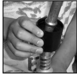
9. Disassemble the interlock guide. Remove the top piece by pulling upward and sliding over the spout. Remove the bottom piece by sliding over the spout.
