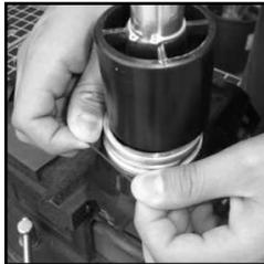
19. Install the new bellows o-ring. Verify that the o-ring seats properly into the machined groove.
