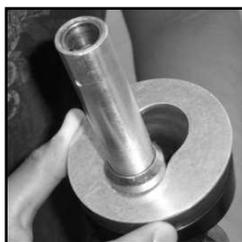
21. Use the bellows retainer plate tool p/n 494712EVR to secure and lock the bellows and boot face in place.
