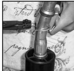
8. Locate the snap ring on the spout. Use the snap ring and needle nose pliers to remove the snap ring from the machined groove. Slide the snap ring upward.
