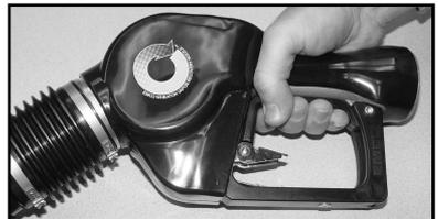
29. Functional test the insertion interlock of the A4005EVR nozzle by compressing the bellows and then squeezing the lever. The A4005EVR nozzle will not function unless the insertion interlock is properly engaged.
