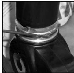
7. Use the scribe tool to remove the bellows o-ring.
