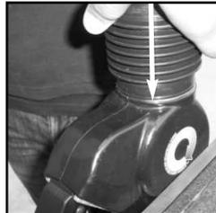
20. Slide the bellows over the spout until the end reaches the nozzle body. Push down over the bellows o-ring until properly seated.
