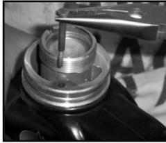
13. Use the needle nose pliers to install the new interlock push rod.
