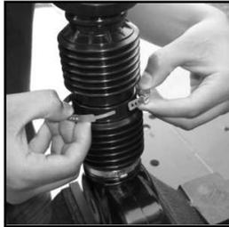
4. Locate the top bellows band clamp. Use the flat head screw driver to dislodge the locking mechanism and remove the band clamp from the bellows.
