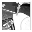
7. Remove the A4005EVR nozzle from the bench vise and place on a flat surface. Use the 1/8" diameter punch and hammer to lightly tap and remove both mounting rivets located on the lever guard.
