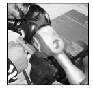
4. Pull the rear end of the scuff guard over the nozzle body unit the dust plug is visible. Use the bench vise to properly secure the A4005EVR nozzle during service.
