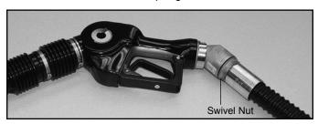
3. It is necessary to remove the A4005EVR nozzle from the A4110EVR hose swivel during the removal and installation of the latch. Use the pipe wrench with flat jaws to loosen the swivel nut. Unfasten the swivel nut by hand from the A4005EVR nozzle to avoid cross threading.
