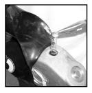
6. Use the flat head screw driver to loosen the brass screw. Use the needle nose pliers to remove the brass screw and spring from the nozzle body.
