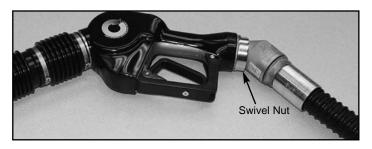
3. It is necessary to remove the A4005EVR nozzle from the A4110EVR hose swivel during the removal and installation of the scuff guard. Use the pipe wrench with flat jaws to loosen the swivel nut. Unfasten the swivel nut by hand from the A4005EVR nozzle to avoid cross threading.
