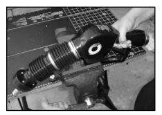
3. It is unnecessary to remove the A4005EVR nozzle from the fueling point during the removal and installation of the boot face. Use the bench vise to properly secure the A4005EVR nozzle during service.
