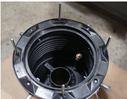
Step 3: Insert (4) 3/8" studs (included) into the holes a minimum of 1/4".
