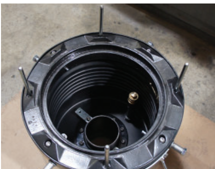
Step 6: Install new rim and seal over studs.
