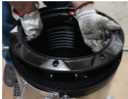
Step 4: Remove remaining 4 bolts. Remove rim and rim seal, and discard both.
