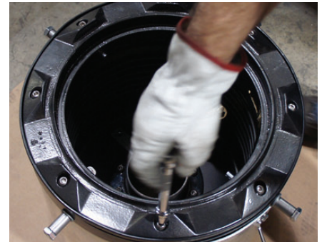
Step 2: Remove every other bolt from the primary rim.
