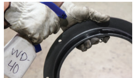
Step 5: Apply lubricant to the new rim seal prior to installing in the primary container.
