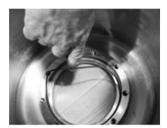
**<u>Step 8:</u>** Install the small cross section o-ring in the groove of the lower flange. Make certain o-ring groove is clean and free of debris.
