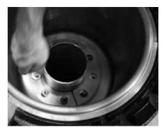
**<u>Step 12:</u>** Hand tighten all nine bolts, ensuring that the bucket is completely down and flat on the rim.
