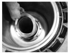
**<u>Step 9:</u>** Install the offset ring, aligning large section of flange with largest open area around the nipple.
