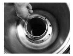
**<u>Step 10:</u>** Install the large cross section o-ring.
