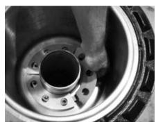
**<u>Step 11:</u>** Install the three flanges using the nine supplied stainless steel bolts and washers. Ensure that the flanges are tight against the nipple.
