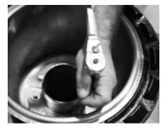
**<u>Step 13:</u>** Using a 9/16" socket, tighten each of the nine bolts to 15 ft. lbs. Pressure may need to be applied to ensure the liner does not shift while tightening bolts.
