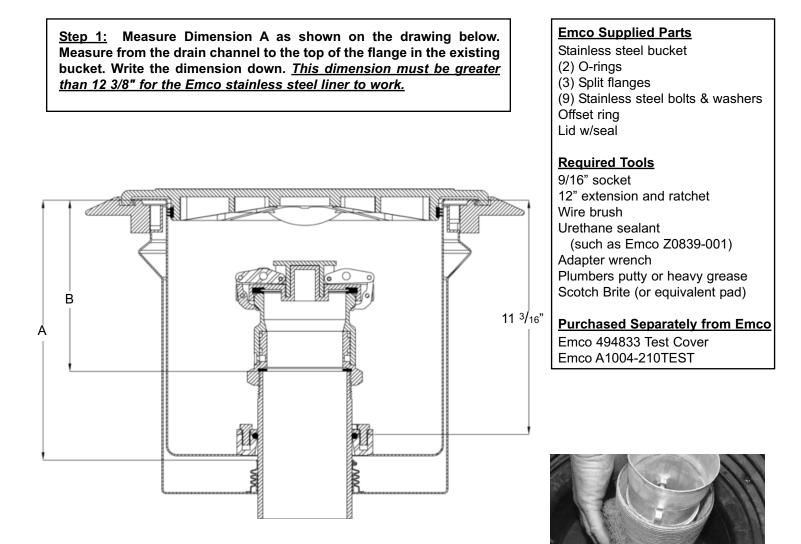
**Step 2:** Measure Dimension B from inside the rim (see drawing above) to the top of the existing nipple. This dimension must be greater than 6 3/4" for a vapor application and 6 1/4" for a fill application (using Emco swivel adapters). If the dimensions are less than specified, an alternative nipple, or a low profile cap and/or adapter will be required. May require use of a non-swivel adapter.
