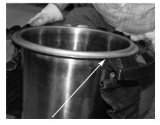
**Step 9:** Test fit the new stainless steel bucket to ensure that it sits completely flat on the top of the rim surface, then remove the stainless steel bucket.
