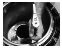
**<u>Step 17</u>:** Using a 9/16" socket, tighten each of the nine bolts to 15 ft. lbs. Pressure may need to be applied to ensure the liner does not shift while tightening bolts.
