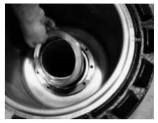
**<u>Step 13:</u>** Install the offset ring, aligning large section of flange with largest open area around the nipple.
