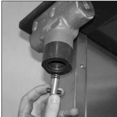
1. Install the adapter plug into the existing splitter valve.
