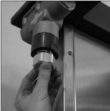
2. Install the adapter nut into the splitter valve.
