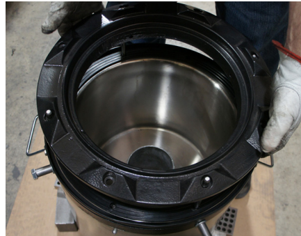
Step 23: Install the second new rim gasket and then place primary rim over studs.
