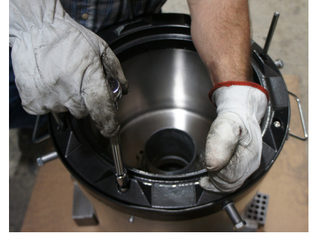
Step 24: Loosely install (4) 3/8" x 1" bolts into open holes in rim.
