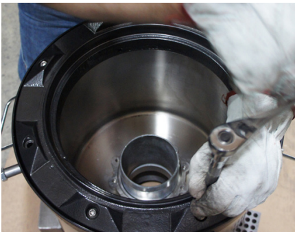
Step 25: Remove studs and replace with the 4 remaining 3/8" x 1" bolts. Tighten all 8 bolts to 20 ft. lbs., alternating in a star pattern.
