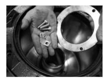
4. Remove all three bolts, washers, grounding clip, ring flange and seal. If necessary, insert one bolt into the threaded hole and use it to break the flange loose.
