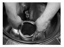
5. Lubricate the inside diameter of the new gasket seal with petroleum jelly or suitable lubricant. Install the new gasket seal.
