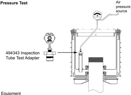
Emco 494343 Inspection Tube Test Adapter (Procured separately from spill containment) Air pressure gauge, scale 0-10 psi Soap solution
