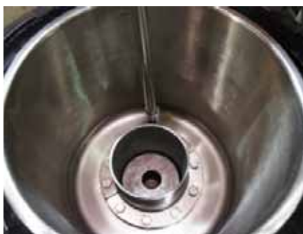
Step 12: Using a \frac{9}{16} " socket, tighten each of the ten bolts to 15 ft. lbs.
