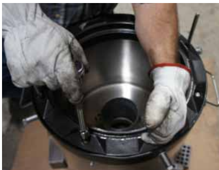
Step 8: Loosely install 4 of the new \frac{3}{8} " x 1" bolts into open holes in rim.
