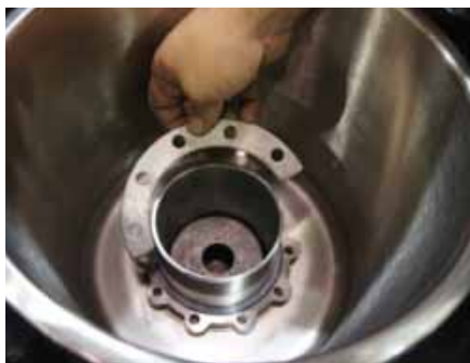
Step 11: Install the two split flanges using the ten supplied stainless steel bolts. Hand tighten all ten bolts, ensuring that the bucket is completely down and flat on the rim.
