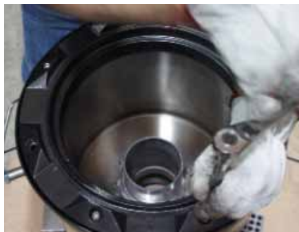
Step 9: Remove studs and replace with the 4 remaining \frac{3}{8} " x 1" bolts. Tighten all 8 bolts to 20 ft. lbs.
