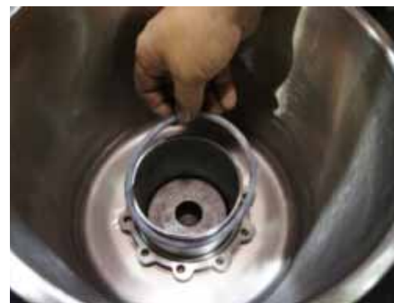
Step 10: Install new o-ring over the nipple, seating it completely in the groove in the stainless steel flange.
