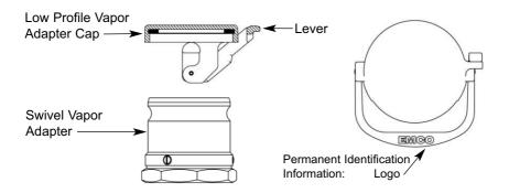
Locate the low profile vapor adapter cap over the swivel vapor adapter and lock into place by pressing down on the lever.
