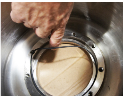
Step 13: Install the small cross section o-ring in the groove of the lower flange. Make certain o-ring groove is clean and free of debris.
