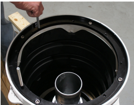
Step 10: Install the 4 studs into 4 of the tapped holes using every other hole.
