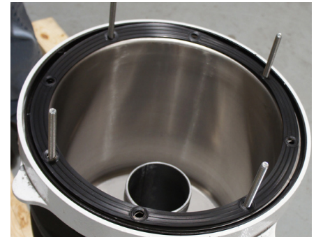
Step 12: Place new bellows gasket onto lip of secondary unit, using studs to assist with alignment.
