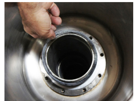
Step 15: Install the large cross section o-ring on top of the aluminum offset ring.
