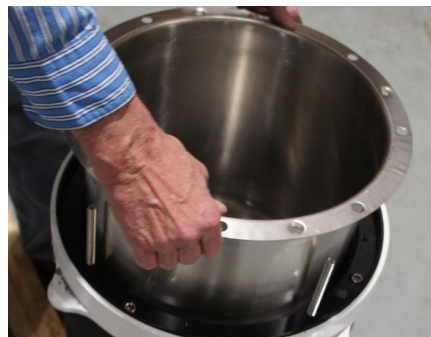
Step 11: Install the secondary unit, using studs to assist with alignment.
