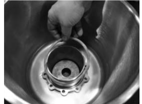
Step 10: Install new o-ring over the nipple, seating it completely in the groove in the stainless steel flange.
