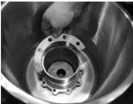
Step 11: Install the two split flanges using the ten bolts. Hand tighten all ten bolts, ensuring that the bucket is completely down and flat on the rim.
