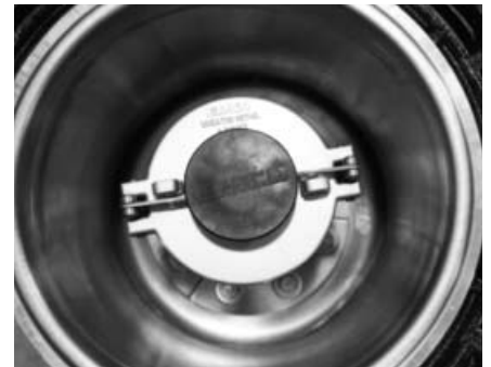
Step 13: Install adapter and cap per instructions included with each.
