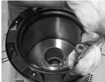
Step 9: Remove studs and replace with the 4 remaining 3/8" x 1" bolts. Tighten all 8 bolts to 20 ft. lbs.
