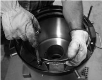
Step 8: Loosely install 4 of the 3/8" x 1" bolts into open holes in rim.
