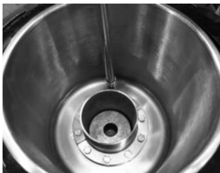
Step 12: Using a 9/16" socket, tighten each of the ten bolts to 15 ft. lbs.
