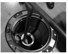
**<u>Step 8</u>**: Install the new primary bellows using the A0081-001H to tighten lining up the holes in the primary bellows with the rim holes in the secondary bellows.
