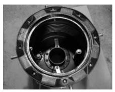
**<u>Step 1:</u>** Remove lid, cap, adapter and dipstick or gauge. Disconnect drain chain. If date and model number tags are present, remove and set aside.
