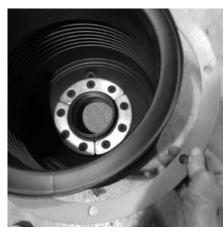
**<u>Step 6:</u>** Slide both bellows support ring segments underneath the secondary bellows, lining up holes in the secondary bellows. The longer bolts may be required.
