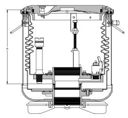
**Step 4:** Measure from grade down to the top of the secondary flange as shown by dimension "A" above. If dimension A is greater than 13", install A0031-175K Riser Extension included with the kit. <u>Do Not</u> use pipe dope on either set of threads.
