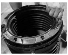
**Step 6:** If bellows is compressed, use the (2) jack bolts to pull the primary rim down to the secondary rim.
