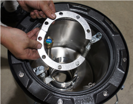
Step 7: Install the 2 split flanges, using 7 of the 8 bolts.
