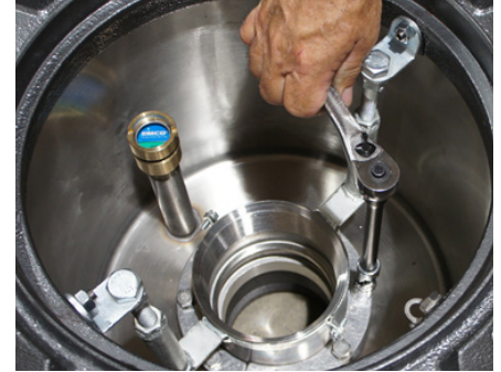
Step 9: Use a 9/16" socket to tighten the bolts to 15 ft. lbs. Note that the flange bolts must be tightened for the interstitial space to pass leak testing.
