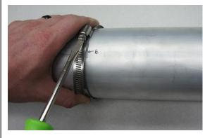
**Step 2:** cut the drop tube at the mark using a fine tooth hacksaw. A hose clamp can be used as a guide if available.
