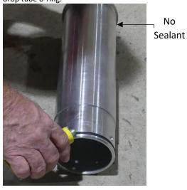
**Step 2:** slide the collar inside the top end of the drop tube and align the four holes. This will be a tight fit. If necessary use a wooden block across the collar to tap into place.
