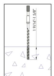
**Step 4:** Clean holes of all debris. Use the following QR Code to see manufacturer installation instructions for typical threaded concrete anchors.
