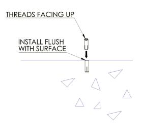
**Step 6:** Insert the setting tool (EMCO 574679) into the anchor and strike with a hammer until the lip of the setting tool meets the top of the anchor (EMCO 574678).
