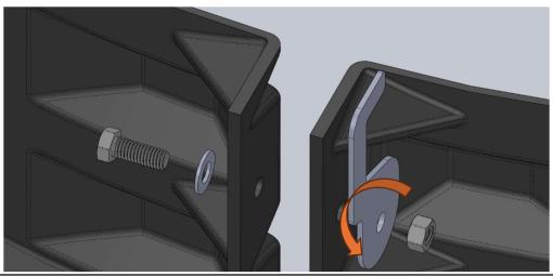
Step 4: Use 1 ea. bolt + 2 ea. washer + 1 ea. nut on bottom hole. Tighten nut.
