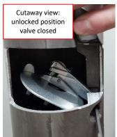
**Step 8:** Re-insert the plug into the valve with the 1/8" allen wrench. Securely tighten.
