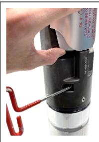
Step 4: Lift up the bottom float as shown and turn the 9/64" allen wrench 90° counterclockwise placing the primary flapper in the unlocked position (valve closed). Release the float but hold the allen wrench in the turned position.
