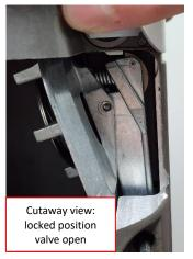
**Step 7:** Re-insert the 9/64" allen wrench. Without moving the float, attempt to turn the wrench counterclockwise to check if the flapper is in the locked open position. If the primary flapper moves less than 5 degrees, then the valve is in proper working order.
