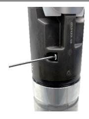
**Step 2:** Using an 1/8" allen wrench, remove the plug from the valve.
