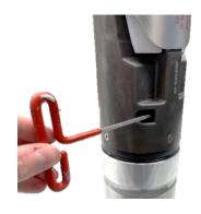
Step 3: Turn the primary flapper counterclockwise with a 9/64" allen wrench. If the wrench turns 5° or less, the primary flapper is in the locked position (valve open) and is working properly.
